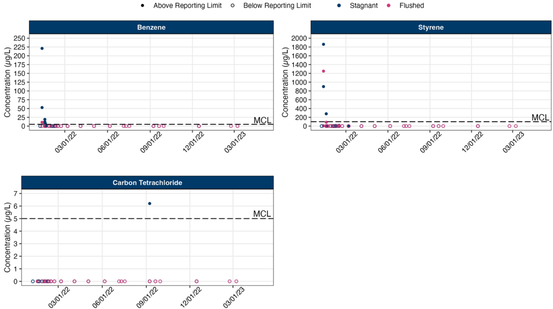
Figure 12. Contaminants detected above the MCL in distribution system sampling
